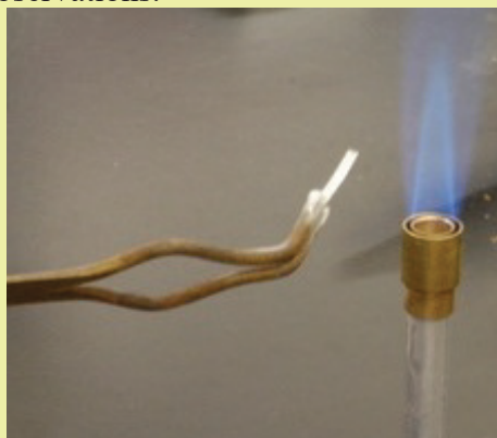
Figure 3.1. Burning of magnesium in air
