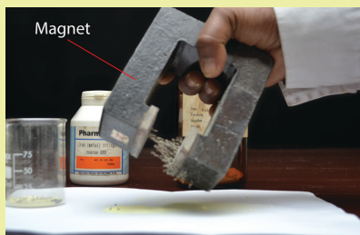
Figure 2.7. A) mixture of iron and sulphur B) Magnetic separation the mixture
