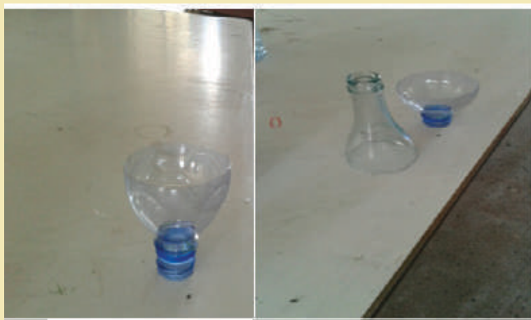
Figure 1.1. Making a Plastic Funnel
