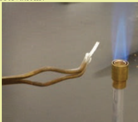
Figure 3.1. Burning of magnesium in air
